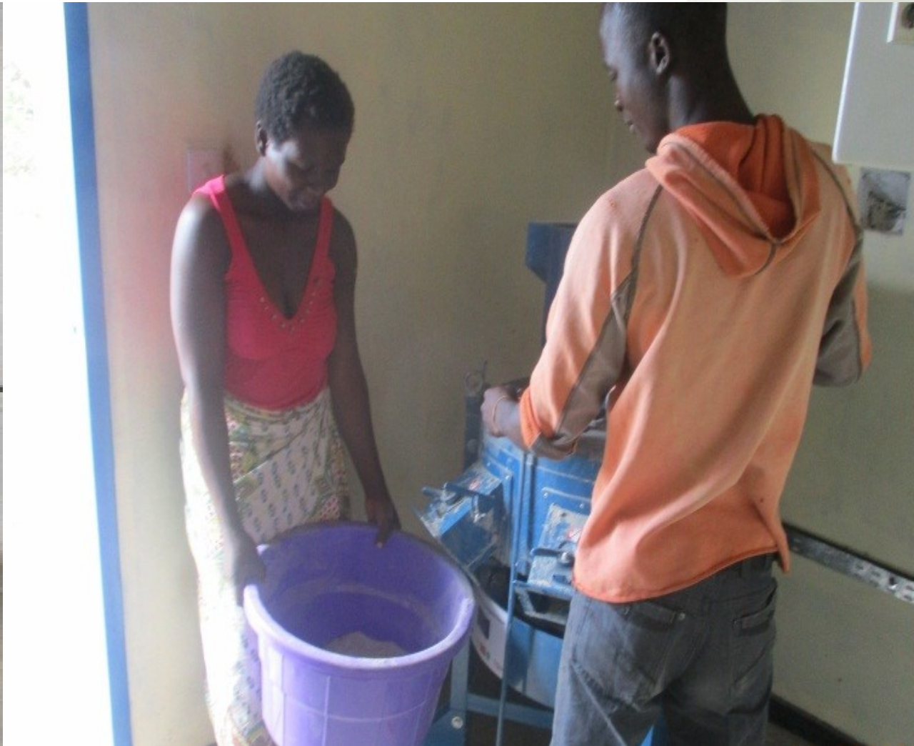
Installed Solar mill and an operator helping a woman grind her maize at Chimombo solar power station
